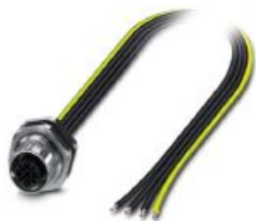
Flush-type connector, Power, 4-position, Socket, M12, S power, Rear mounting, M16 x 1.5, Individual wires, cable length: 0.5 m, 1.31 mm 2 , UL/cUL stranded hook-up wire
