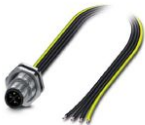
Flush-type connector, Power, 4-position, Plug, M12, S power, Rear mounting, M16 x 1.5, Individual wires, cable length: 0.5 m, 1.31 mm 2 , UL/cUL stranded hook-up wire
