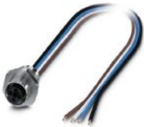
Flush-type connector, Power, 4-position, Socket, M12, T power, Front mounting, M16 x 1.5, Individual wires, cable length: 0.5 m, 1.31 mm 2 , UL/cUL stranded hook-up wire
