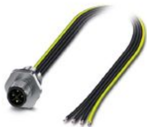
Flush-type connector, Power, 4-position, Plug, M12, S power, Front mounting, M16 x 1.5, Individual wires, cable length: 0.5 m, 1.31 mm 2 , UL/cUL stranded hook-up wire
