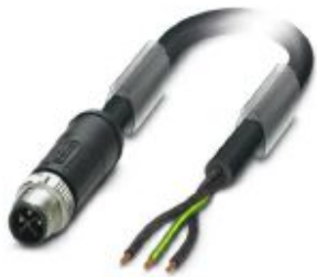
Power cable, 3-position, PVC, black, Plug straight M12, coding: S, on free cable end, cable length: 5 m, for AC current up to 16 A/230 V
