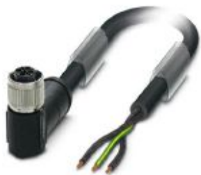
Power cable, 3-position, PVC, black, free cable end, on Socket angled M12, coding: S, cable length: 10 m, for AC current up to 16 A/230 V
