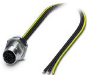
Flush-type connector, Power, 3-position, Socket, M12, S power, Rear mounting, M16 x 1.5, Individual wires, cable length: 0.5 m, 1.31 mm 2 , UL/cUL stranded hook-up wire
