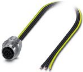
Flush-type connector, Power, 3-position, Socket, M12, S power, Front mounting, M16 x 1.5, Individual wires, cable length: 0.5 m, 1.31 mm 2 , UL/cUL stranded hook-up wire
