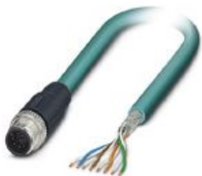
Network cable, Ethernet CAT5 (1 Gbps), 8-position, PUR, Plug straight M12 / IP67, coding: A, on free cable end, cable length: 2 m
