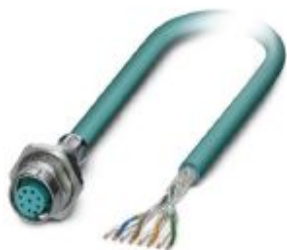
Assembled Ethernet cable, shielded, 4-pair, AWG 26 suitable for drag chain (19-wire), RAL 5021 (sea blue), M12 flush-type socket, rear wall/screw mounting with M16 thread on free cable end, line, length 2 m
