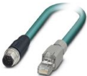
Network cable, Ethernet CAT5 (1 Gbps), 8-position, PUR, Plug straight M12 / IP67, coding: A, on Plug straight RJ45 / IP20, cable length: 2 m
