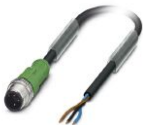
Sensor/actuator cable, 3-position, PVC, black RAL 9005, Plug straight M12, coding: A, on free cable end, cable length: 1.5 m
