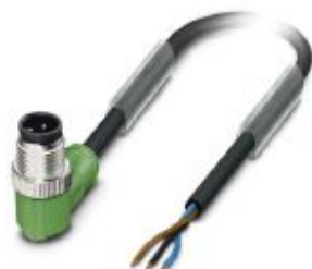
Sensor/actuator cable, 3-position, PVC, black RAL 9005, Plug angled M12, coding: A, on free cable end, cable length: 3 m
