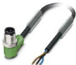
Sensor/actuator cable, 3-position, PVC, black RAL 9005, Plug angled M12, coding: A, on free cable end, cable length: 5 m
