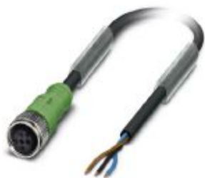
Sensor/actuator cable, 3-position, PVC, black RAL 9005, free cable end, on Socket straight M12, coding: A, cable length: 3 m
