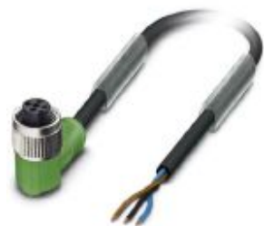
Sensor/actuator cable, 3-position, PVC, black RAL 9005, free cable end, on Socket angled M12, coding: A, cable length: 3 m
