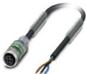
Sensor/actuator cable, 3-position, PVC, black RAL 9005, free cable end, on Socket straight M12, coding: A, with 2 LEDs, cable length: 10 m
