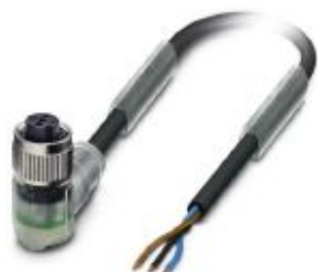
Sensor/actuator cable, 3-position, PVC, black RAL 9005, free cable end, on Socket angled M12, coding: A, with 2 LEDs, cable length: 10 m
