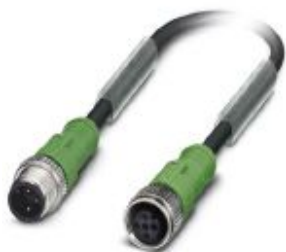
Sensor/actuator cable, 3-position, PVC, black RAL 9005, Plug straight M12, coding: A, on Socket straight M12, coding: A, cable length: 0.6 m
