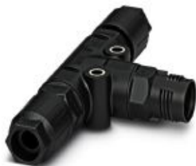
T distributor, QUICKON connection, number of positions: 3+PE, 0.5 mm 2 ... 1.5 mm 2 , 690 V, 17.5 A, black, With two QUICKON nuts, cable diameter range: 5 mm ... 9.5 mm
