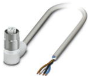
Sensor/actuator cable, 4-position, PP-EPDM halogen-free, gray RAL 7035, free cable end, on Socket angled M12, A-coded, cable length: 15 m, Hygienic design, with high-grade steel knurl
