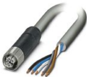
Power cable, 5-position, PVC, gray RAL 7001, Socket straight M12, coding: L, on free cable end, cable length: 3 m, for direct current up to 16 A/63 V
