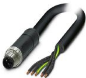
Power cable, 5-position, PVC, black-gray RAL 7021, Plug straight M12, coding: K, on free cable end, cable length: 3 m, for AC current up to 16 A/690 V
