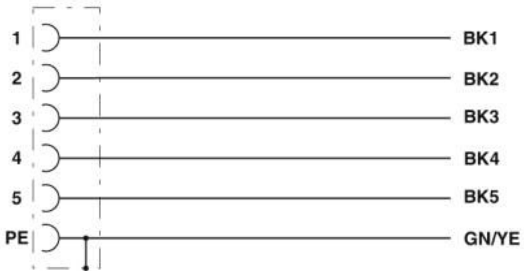
Contact assignment of the M12 socket
