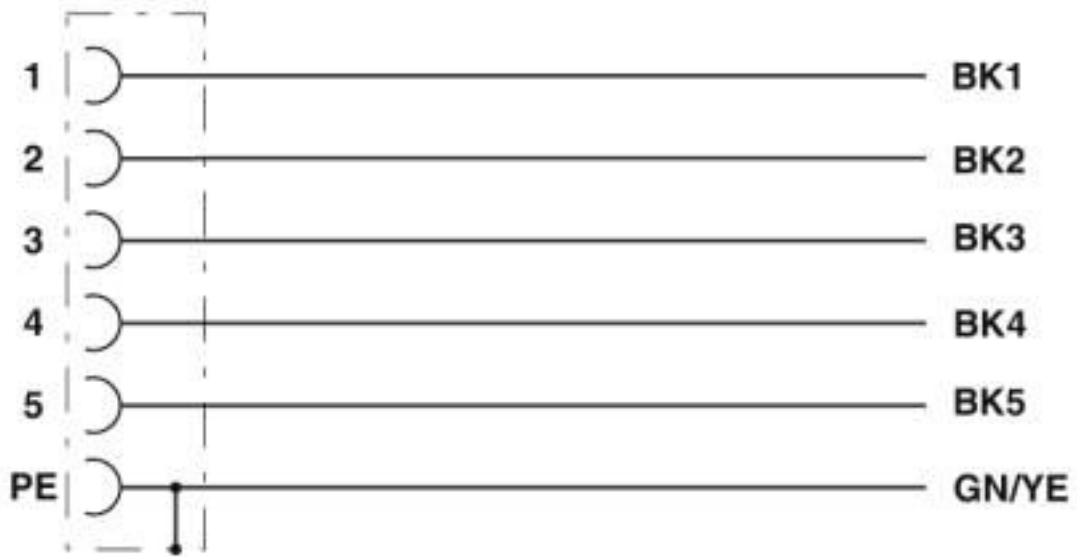
Contact assignment of the M12 socket
