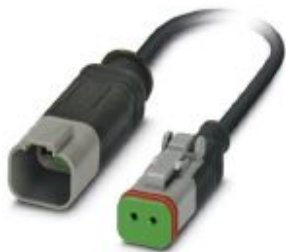
Sensor/actuator cable, 2-position, PUR halogen-free, black-gray RAL 7021, Plug straight DEUTSCH DT04-2P Clip locking, on Socket straight DEUTSCH DT06-2S Clip locking, cable length: 0.3 m
