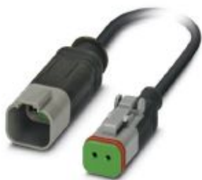
Sensor/actuator cable, 2-position, PUR halogen-free, black-gray RAL 7021, Plug straight DEUTSCH DT04-2P Clip locking, on Socket straight DEUTSCH DT06-2S Clip locking, cable length: 1.5 m
