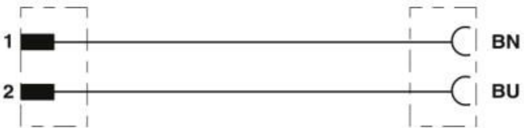
Contact assignment of the DEUTSCH connectors
