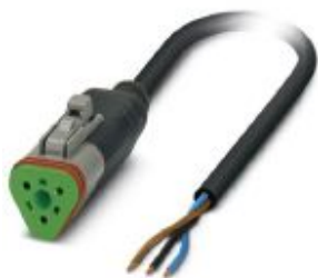
Sensor/actuator cable, 3-position, PUR halogen-free, black-gray RAL 7021, free cable end, on Socket straight DEUTSCH DT06-3S Clip locking, cable length: 3 m
