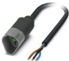
Sensor/actuator cable, 3-position, PUR halogen-free, black-gray RAL 7021, Plug straight DEUTSCH DT04-3P Clip locking, on free cable end, cable length: 1.5 m
