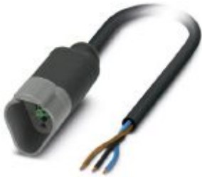
Sensor/actuator cable, 3-position, PUR halogen-free, black-gray RAL 7021, Plug straight DEUTSCH DT04-3P Clip locking, on free cable end, cable length: 5 m
