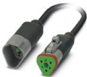
Sensor/actuator cable, 3-position, PUR halogen-free, black-gray RAL 7021, Plug straight DEUTSCH DT04-3P Clip locking, on Socket straight DEUTSCH DT06-3S Clip locking, cable length: 0.3 m
