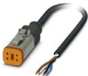
Sensor/actuator cable, 4-position, PUR halogen-free, black-gray RAL 7021, free cable end, on Socket straight DEUTSCH DT06-4S Clip locking, cable length: 10 m
