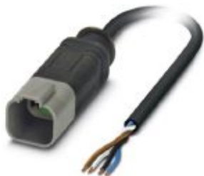
Sensor/actuator cable, 4-position, PUR halogen-free, black-gray RAL 7021, Plug straight DEUTSCH DT04-4P Clip locking, on free cable end, cable length: 10 m
