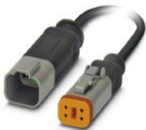
Sensor/actuator cable, 4-position, PUR halogen-free, black-gray RAL 7021, Plug straight DEUTSCH DT04-4P Clip locking, on Socket straight DEUTSCH DT06-4S Clip locking, cable length: 0.3 m
