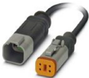
Sensor/actuator cable, 4-position, PUR halogen-free, black-gray RAL 7021, Plug straight DEUTSCH DT04-4P Clip locking, on Socket straight DEUTSCH DT06-4S Clip locking, cable length: 1.5 m
