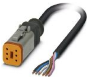
Sensor/actuator cable, 6-position, PUR halogen-free, black-gray RAL 7021, free cable end, on Socket straight DEUTSCH DT06-6S Clip locking, cable length: 3 m
