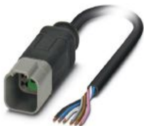
Sensor/actuator cable, 6-position, PUR halogen-free, black-gray RAL 7021, Plug straight DEUTSCH DT04-6P Clip locking, on free cable end, cable length: 1.5 m
