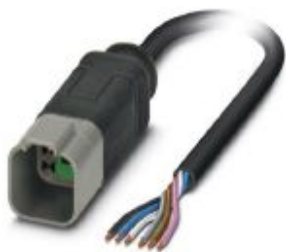
Sensor/actuator cable, 6-position, PUR halogen-free, black-gray RAL 7021, Plug straight DEUTSCH DT04-6P Clip locking, on free cable end, cable length: 5 m
