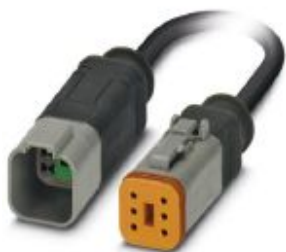
Sensor/actuator cable, 6-position, PUR halogen-free, black-gray RAL 7021, Plug straight DEUTSCH DT04-6P Clip locking, on Socket straight DEUTSCH DT06-6S Clip locking, cable length: 1.5 m
