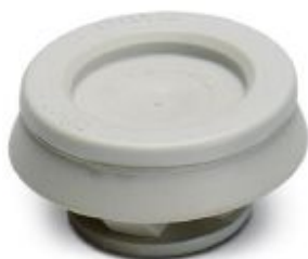
Membrane screw connection, cable gland material: Polypropylene, external cable diameter 4 mm ... 10 mm, shielding: no, connecting thread: M16, color: light gray
