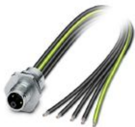
Flush-type connector, Power, 5-position, Plug, M12, K - Power, Front mounting, M16 x 1.5, Individual wires, cable length: 0.2 m, 2.50 mm 2 , PEX litz wire
