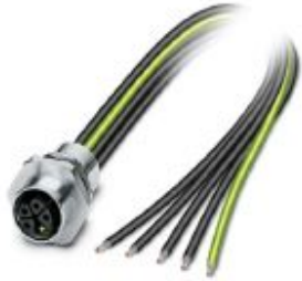
Flush-type connector, Power, 5-position, Socket, M12, K - Power, Front mounting, M16 x 1.5, Individual wires, cable length: 0.2 m, 2.50 mm 2 , PEX litz wire
