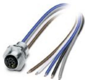
Flush-type connector, Power, 5-position, Socket, M12, L - Power, Front mounting, M16 x 1.5, Individual wires, cable length: 0.2 m, 2.50 mm 2 , PEX litz wire
