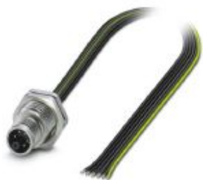
Flush-type connector, Power, 6-position, Plug, M12, M - Power, Rear mounting, M16 x 1.5, Individual wires, cable length: 0.2 m, 1.31 mm 2 , UL/cUL stranded hook-up wire
