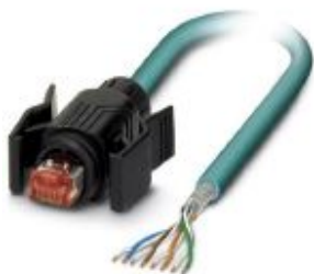
Assembled Ethernet cable, CAT6, shielded, 4-pair, AWG 26 stranded (7-wire), RAL 5021 (water blue), RJ45 plug/IP67, black on free conductor end, line, length 5 m
