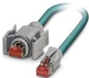
Assembled Ethernet cable, CAT6, shielded, 4-pair, AWG 26 stranded (7-wire), RAL 5021 (water blue), RJ45 plug/IP67, gray on RJ45 plug/IP20, line, length 5 m
