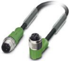
Sensor/actuator cable, 3-position, PVC, black RAL 9005, Plug straight M12, coding: A, on Socket angled M12, coding: A, cable length: 3 m
