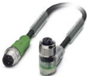
Sensor/actuator cable, 3-position, PVC, black RAL 9005, Plug straight M12, coding: A, on Socket angled M12, coding: A, with 2 LEDs, cable length: 0.3 m
