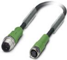
Sensor/actuator cable, 3-position, PVC, black RAL 9005, Plug straight M12, coding: A, on Socket straight M8, cable length: 1.5 m
